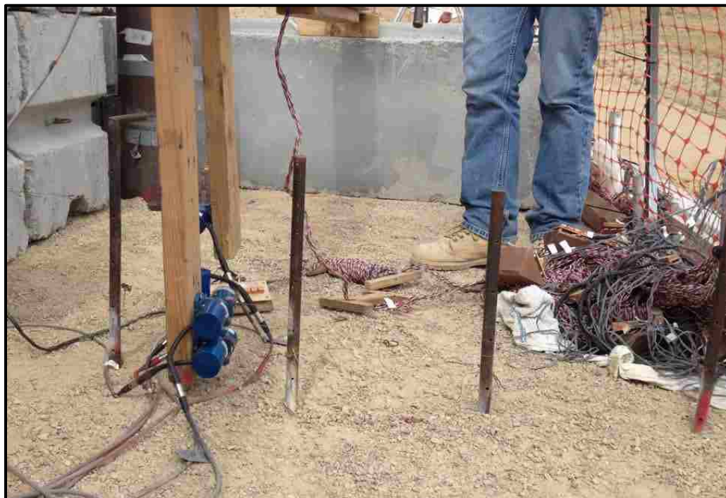
Figure 4-2: Horizontal ground displacement setup.
